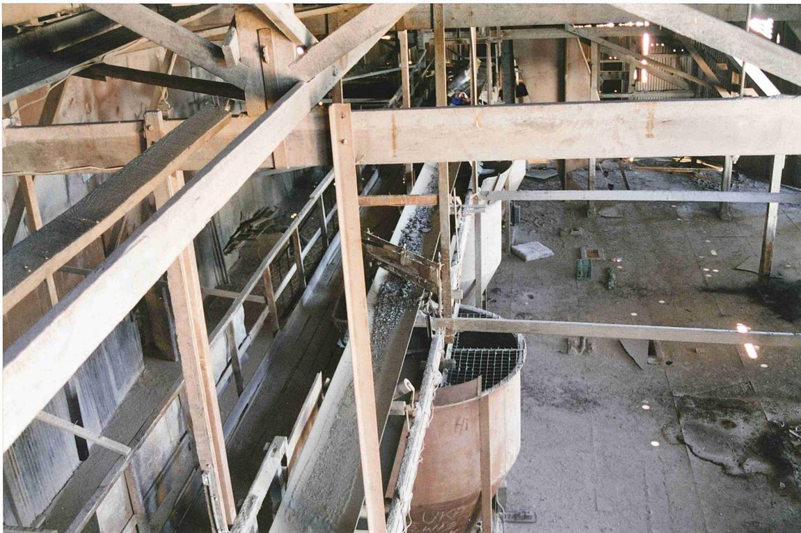
Figure 17. Building 5 - mezzanine level. Photograph shows the conveyor belt used to deposit material into the hoppers situated on the first floor.
