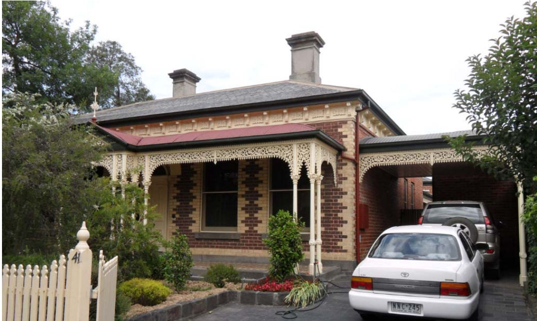
Figure 7. 41 Dixon Street, showing the carport on the north side which employs simplified versions of the verandah posts and frieze. (source: Context 2016)
