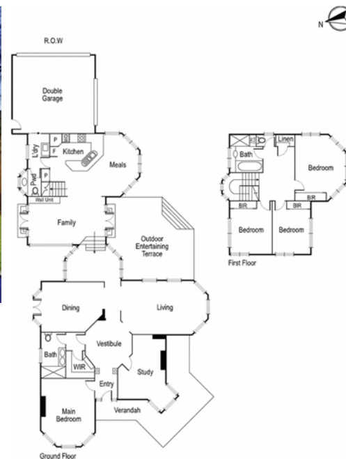
Figure 8. Floor plan of 44 Elizabeth Street, Malvern depicting the octagonal vestibule connecting the various projecting bays (source: Realestate.com.au, c2010).
