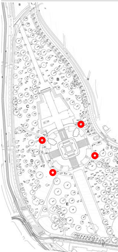
Figure 107 Plan showing the locations of the light pylons (marked by the red circles).
