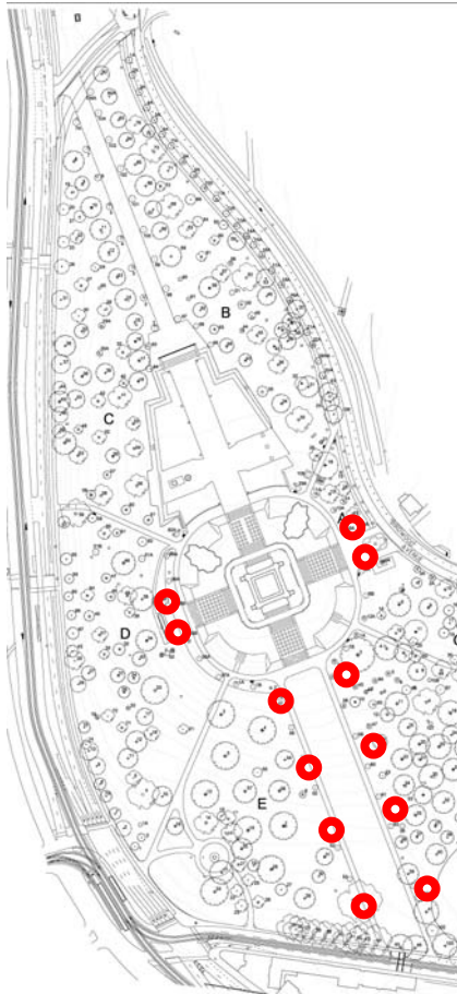
Figure 109 Plan showing the approximate locations of the cast iron lamp posts (marked by the red circles).
