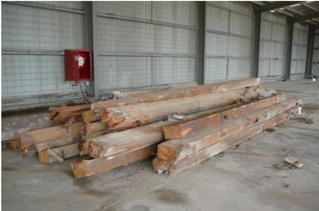
Figure 2 Collection of oregon beams and rafters retained from Sheds 4 - 6.
